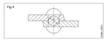
Rivet cross-section is the hole cross-section.
